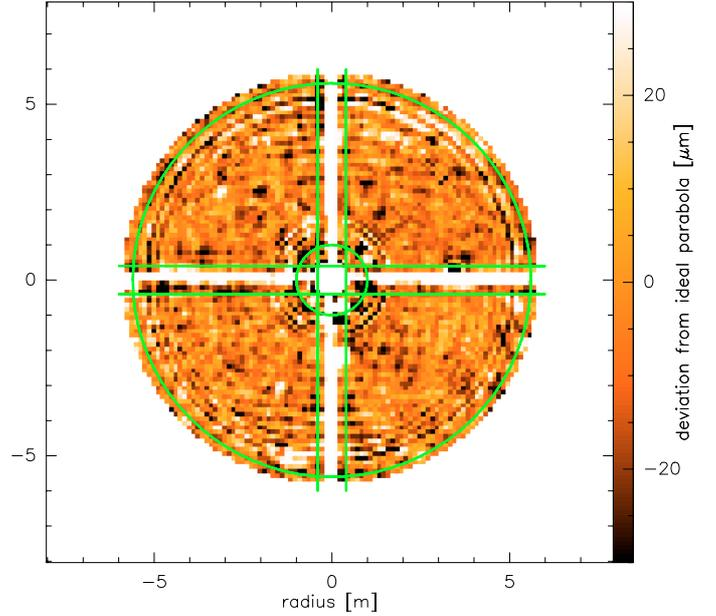
**Fig. 3.** The surface error pattern of the APEX main reflector after the April 2005 holography session. Masking the inner 1 m and the projected area of the quadrupod legs, but without radial tapering, the surface accuracy is determined to be  $14.7 \mu\text{m}$  rms.
