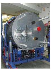
It contains a new 18/21cmsystem (for continuum, pulsar and spectroscopy, VLBI observations), as well two as spectroscopy (1.9cm receivers and 1.0cm). In addition, a 2.5cm-receiver for holography of the reflector is included. Switching the individual between systems is done by rotating and shifting the box into the focus position and can be done within one minute.
