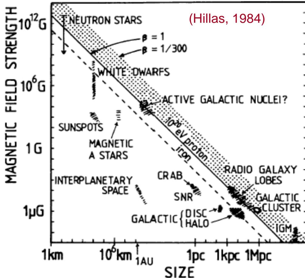
Figure 1 Size and magnetic field strength of possible sites of particle acceleration. Objects below the diagonal line cannot accelerate protons to  $10^{20}\text{ eV}$ .
