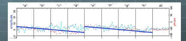
phases adjusted by first tone within band (3.4, 2.4, 1.4, 0.4, 4.4, 3.4, 2.4, 1.4 MHz)
