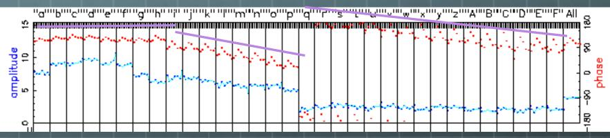
after removal of hand-fitted ionosphere & automatic pcal alignment
