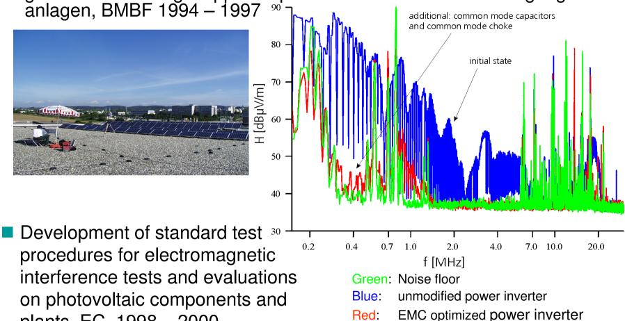
interference tests and evaluations on photovoltaic components and plants, EC, 1998 - 2000
