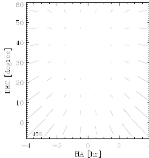
FIG. 4.— The artificial shear pattern induced by the non-coplanar effect, for the case of  $(l, m) = (7', 7')$  away from the phase-tracking center. The line at the bottom-left indicates a distortion of 45%.
