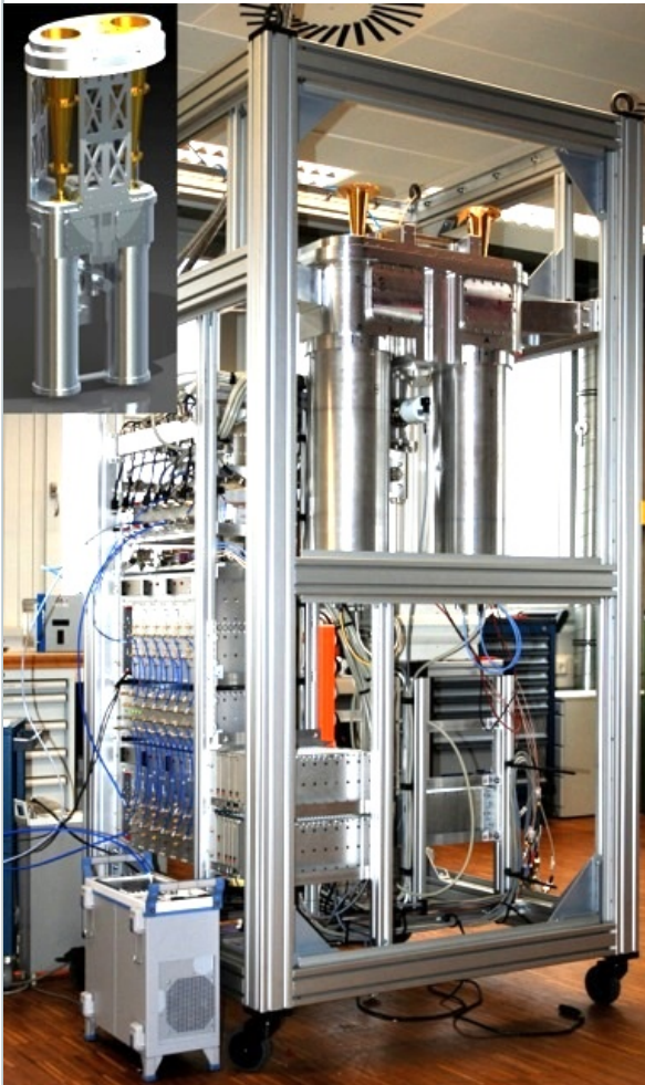
Fig. 1 K-Band frontend during lab commissioning. Space limitations require to remove the feed horns for testing. Small picture: CAD model of the K-Band Receiver incl. the feed horns. Credit to C. Kasemann
