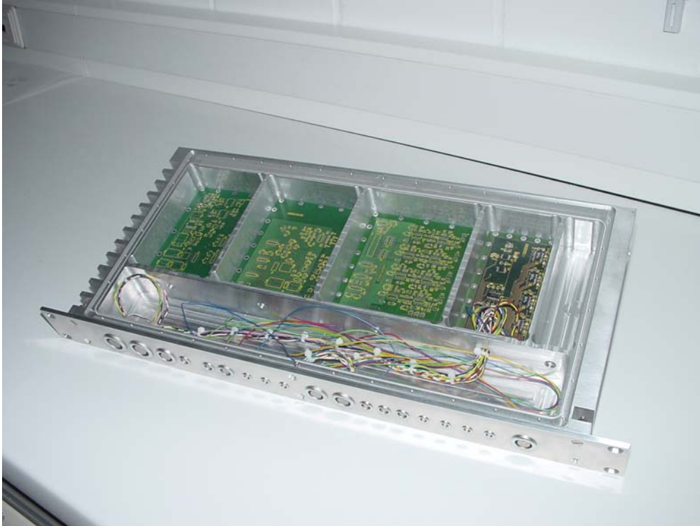
Figure 4-1: Remote controllable analog bias box developed by the MPIfR for the GREAT receiver on SOFIA. This box can be used for mixer bias, B-field, cold amplifier and LO chain multipliers. A local panel with displays is available for work in the receiver cabins.
