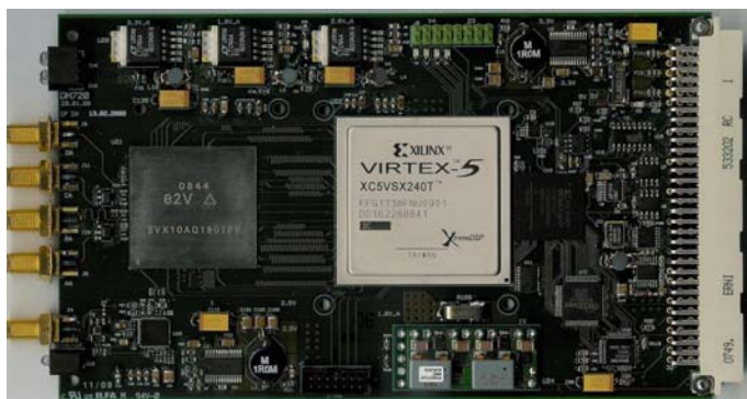
Fig. 3. Currently in lab tests: The new 2.5 GHz bandwidth XFFTS, making use of a first sample of E2V's 5 GS/s 10-bit ADC and the high performance Xilinx Virtex-5 SX240T FPGA.
