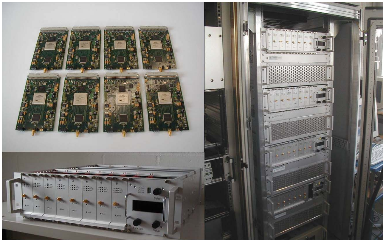
Fig. 1. The APEX wideband AFFTS consists of four FFTS-crates, each equipped with 8 FFTS boards and one FFTS-controller with LCD unit. The frequency resolution (equivalent noise bandwidth) for the standard board configuration with 1.5 GHz bandwidth and 8192 spectral channels per board is 212 kHz.
