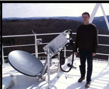
WVR is mounted on Effelsberg focus cabin roof looking skywards along optical axis
