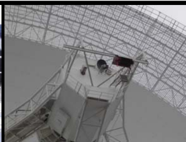
WVR is mounted on Effelsberg focus cabin roof looking skywards along optical axis
