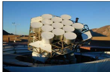
Figure 1: The CBI instrument in its “compact” configuration optimized for polarization measurements (courtesy of R. Bustos).
