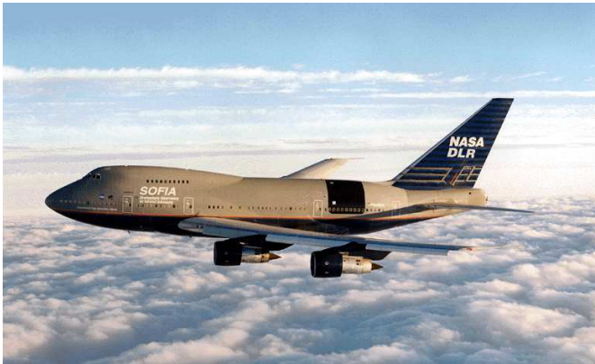
Figure 8: The Boeing 747-SP aircraft which is to be modified to contain a 2.5 m telescope, the Stratospheric Observatory for Infrared Astronomy .
