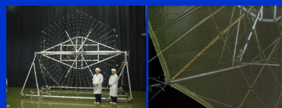
9-m offset cassegrain antenna of seven hexagonal modules (Light weight, Easy adjustment)
