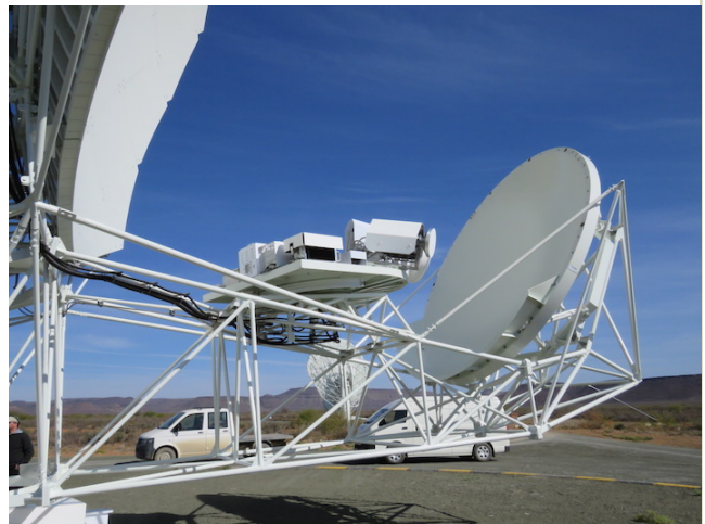
Fig. 1: The S-band receiver installed in the indexer of one of the MeerKAT dishes. A second dish can be seen in the background.
