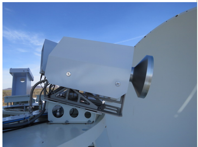
Fig. 2: The S-band receiver with its feed horn.
