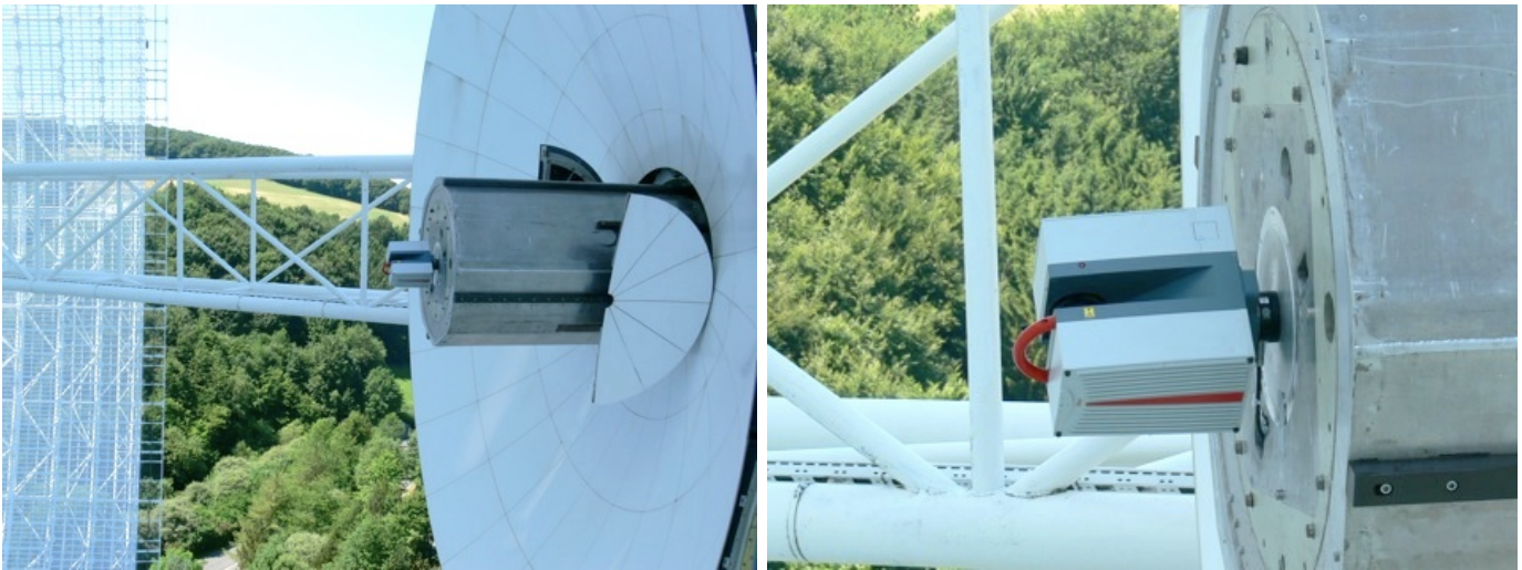
The Leica terrestrial laser scanner in the prime focus of the 100-meter-telescope. It was mounted in an empty receiver box.
